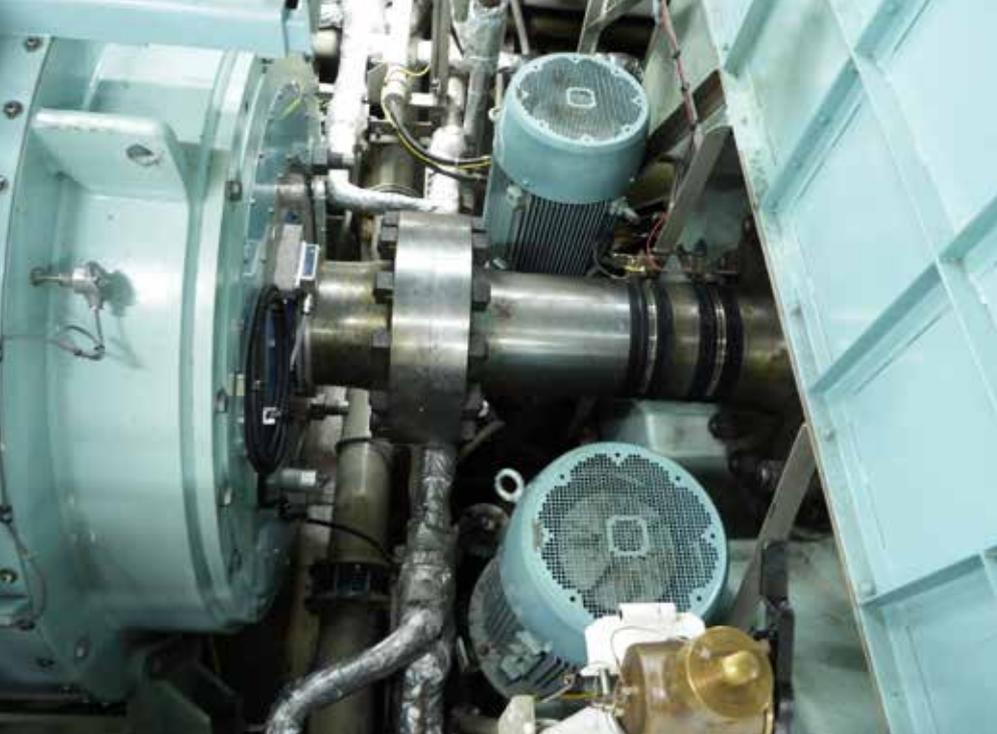
Shows the main engine (right, propulsion shaft and the PTI generator (left)
